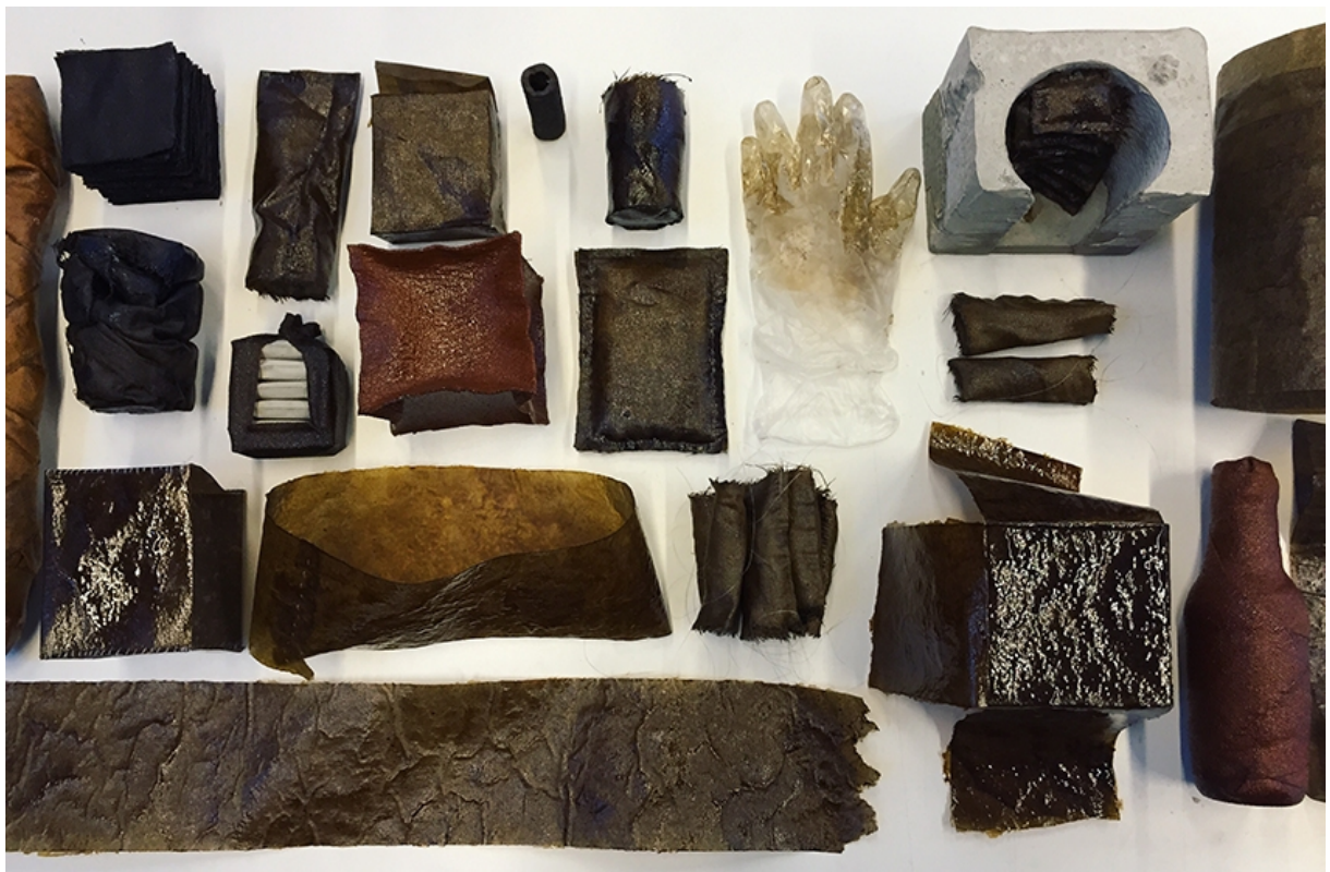
Image 4. Shellac combinations, laid out for comparison and evaluation, sizes between 2x5 cm and 30x30 cm. T.D. 2015-2016
