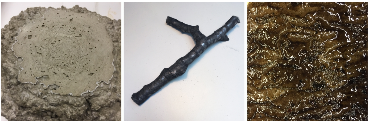
Image 3. Concrete surface (7 cm across), hammered steel wool sewn onto branch (ca 20 cm long) and thick layers of shellac (detail of 7x7 cm test), T.D. 2015-2017
