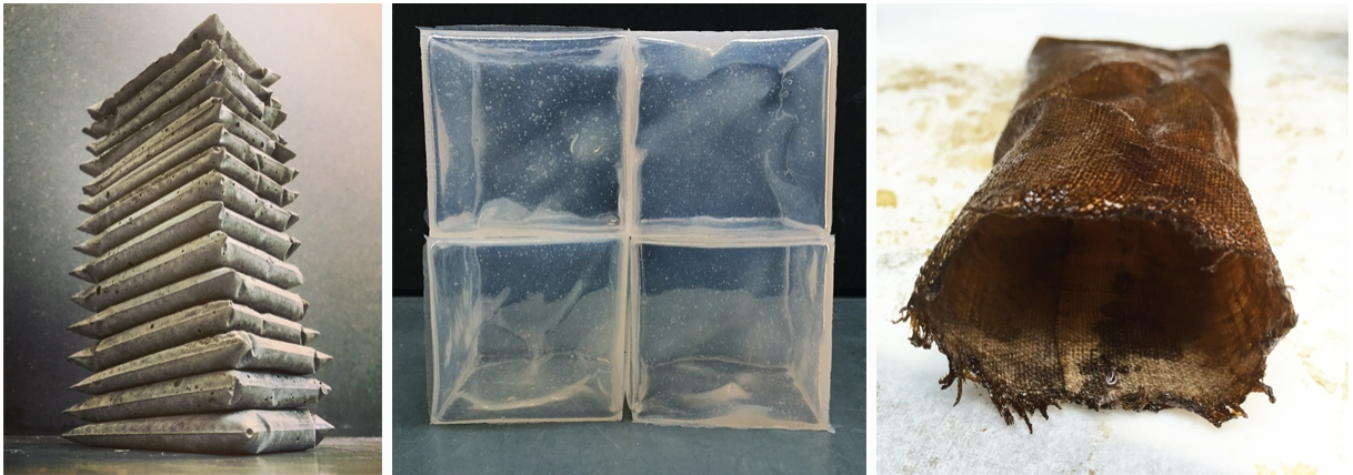
Image 2. Concrete (30x8x5 cm), silicone (20x10x20 cm) and shellac (3x10x5 cm) tests, T.D. 2015-2016
